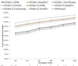
Figure 8. Power saving of the routing algorithms for the number of sensor node = 1000
