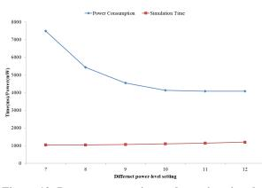
Figure 10. Power consumption and running time by using EEGRA II with different power-level settings.
